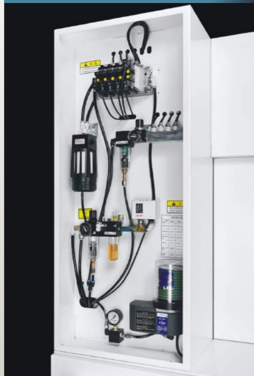
Pneumatic and Lubricant system
