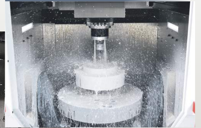
Circular water Flushing System
